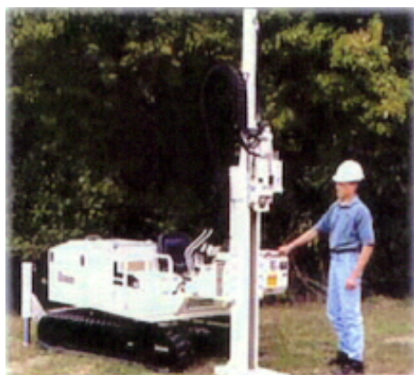
Fig. 3.4 The GeoProbe™ 54DT direct-push mobile rig.
